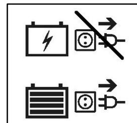
The light emitting diode (LEDs) in the steering unit indicates the remaining capacity of your batteries. If the battery charger is turned on and no LED's are lit, check the fuse. If the red LED does not illuminate, the charger is defective. Consult your specialist dealer.
