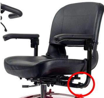
1. Loosen the star knob on the back of the scooter.
