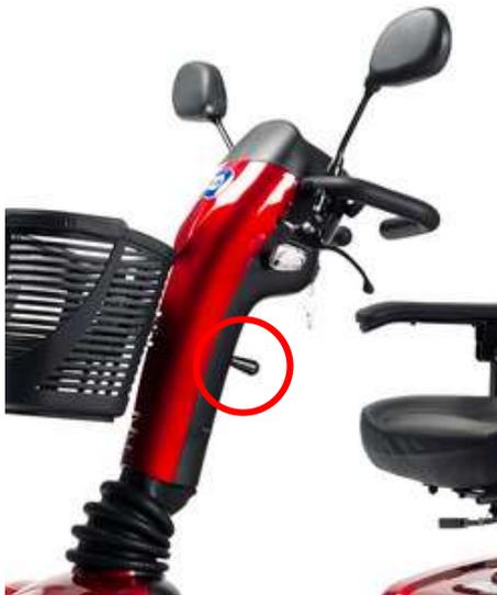
The steering unit can be adjusted to many different positions (stepless) to suit each driver.
