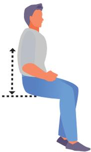
The person is seated on a chair or on a flat surface. Measure the distance between the seat and the middle of the shoulder blades. If the user needs more support, the backrest should be set higher than this measurement. If the person wishes to have a more active position, the backrest height may be lower.
