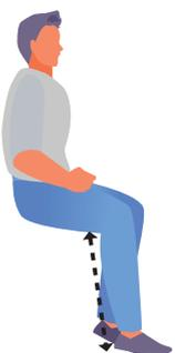
The person is seated on a chair or on a flat surface. Measure the distance between the popliteal fossa (back of the knee) and the heel. Subtract the thickness of the chosen cushion from this measurement.
