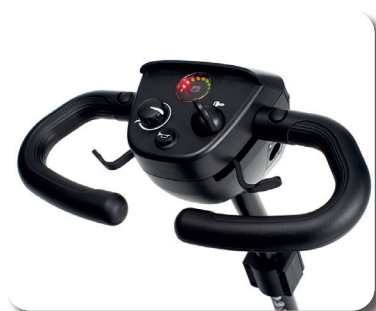
User-friendly controller with a battery status LED indicator
