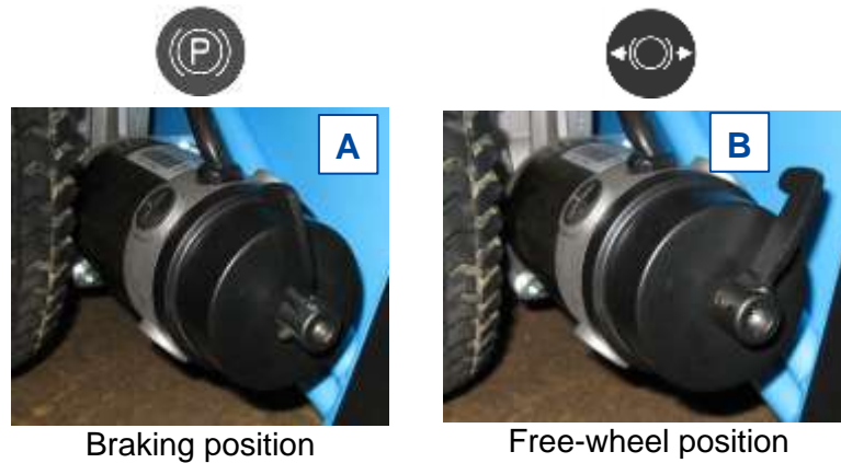
Figure 8 Operating free-wheel lever
