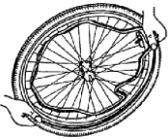
Push the tyre over the edge of the rim, starting behind the air valve. Inflate the tube slightly until it is round, and place it inside the tyre.
