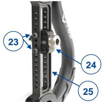
\* The attachment cube has been fitted with four sets of two matching holes. Choose the set that corresponds to the required camber angle as shown in the picture.
