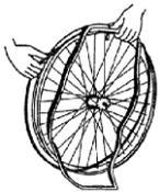
Place the rim belt in position over the air valve before inserting it into the rim. The rim belt can now be pulled over easily. Check that all spoke heads are covered (a rim belt is not required in the case of a plastic rim).
