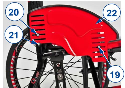
Repeat the adjustments above for the second side plate. Make sure that both side plates are set to the same height and dept, and that they are firmly secured.
