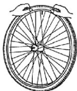
If the tube fits inside the tyre without any folds (in case of folds: let out some air), then the upper side of the tyre can be pressed lightly onto the rim with both hands, starting at the air valve. Lightly push the air valve inwards and pull it out again to make sure that the tyre is positioned properly in the region of the air valve.
