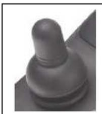
Moving the joystick will drive the electric wheelchair in that direction. The amount of joystick movement will determine the speed that the powerchair will move in that direction.
