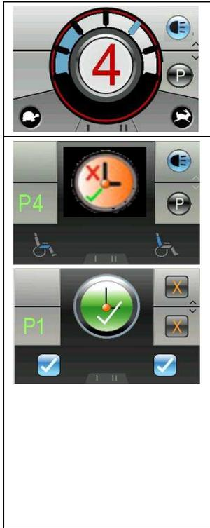
Select the program function using the field selection button (9) and the display will show the menu for the special functions.
