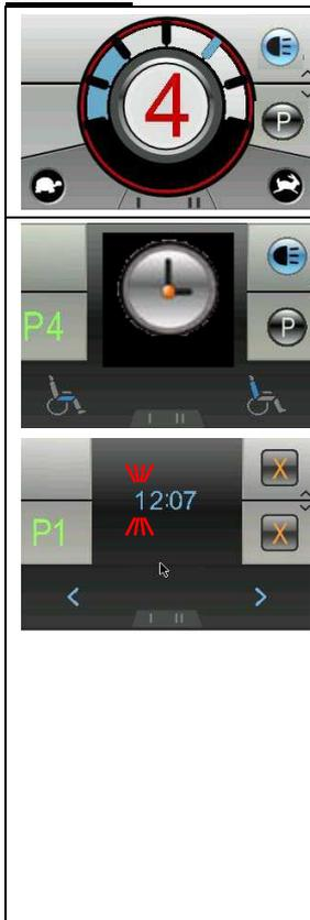
Select the program function using the field selection button (9) and the display will show the menu for the special functions.
