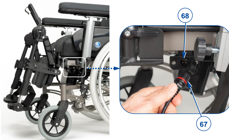
Figure 16 Location of connection point
