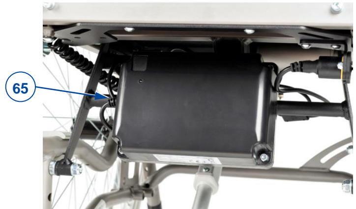
Figure 15 Battery location on wheelchair
