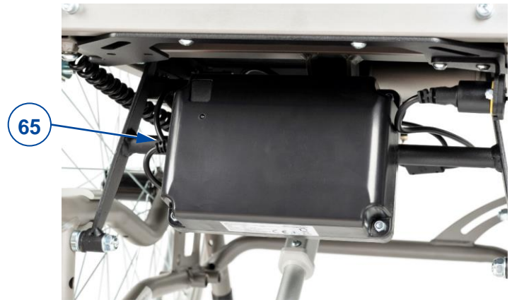
Figure 15 Battery location on wheelchair
